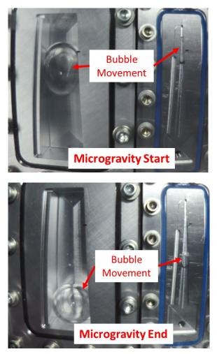
Tapered LAD Bubble Movement in the 2019Suborbital TestIn microgravity, the bubble moved towards thewider end of the channel due to capillary action.
