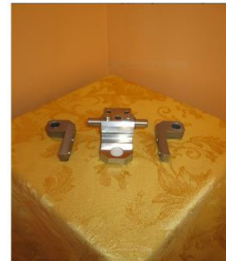
Figure 1: Upper gimbal mount assembly developed for usage on a lunar lander test platform. The test platform was being fabricated for usage by Team Synergy Moon in its bid for the Google Lunar X Prize. A similar mount assembly will be used for future VTVL vehicles.
